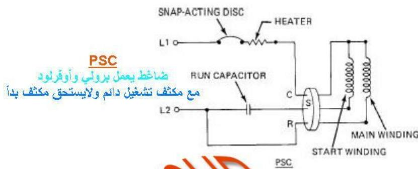
Figure 9.39 Permanent split-capacitor motor schematic. (Courtesy of Tecumseh.)
