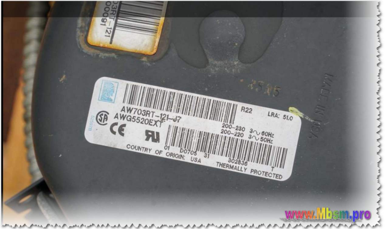
Tecumseh ,Reciprocating ,Compressor, AW703RT-121-J7, AWG5520EXT 200-230/3
